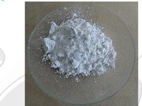
Calcium oxide obtained by thermal decomposition of calcium carbonate at high temperature (above 825 °C).
