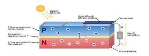
**Photovoltaic cell:** It has a thin metallic layer coated with silver or gold which act as electrode, also has metal base plate which act as another electrode • Two layers are separated by semiconductor layer of selenium, when light radiation falls on selenium layer. • This creates potential diff. between the two electrode and cause flow of current.
