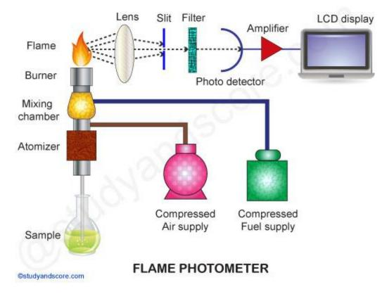
Schematic Representation of the Flame Photometer
