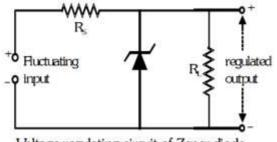
Voltage regulating circuit of Zener diode
