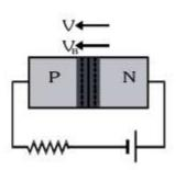
Only minority carriers will drifted. It means the current flow in principally due to minority charge carriers and is very small (in the order of µA). This bias is called as reversed Bias.
