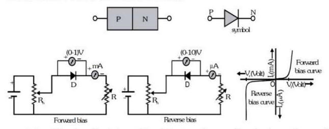
In forward bias when voltage is increased from 0V is steps and corresponding value of current is measured, the curve comes as OB of figure. We may note that current increase very sharply after a certain voltage knee voltage. At this voltage, barrier potential is completely eliminated and diode offers a low resistance.
