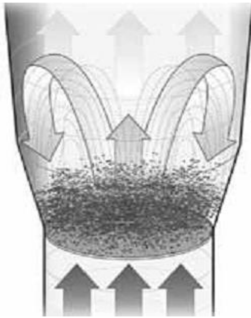
Figure-11. Schematic Fluid bed Dryer
