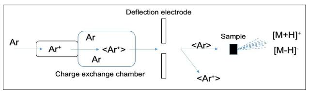
After the sample is ionized, its positive charge product is mostly present in the form of proton bonding or alkali metal ion binding. Generally only a small amount of alkali metal ions are needed, and a  $[M+Na]^+$  or  $[M+K]^+$  signal can appear in the mass spectrometer.
